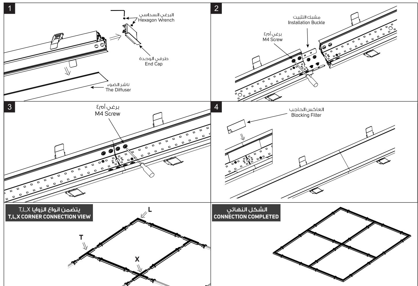
(1): Remove the end cap, then take out the diffuser as per FIG1.
